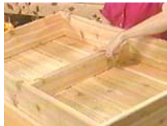
Use a center brace to help support the table top
