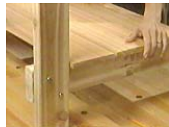
Cut and attach three boards to the supports
