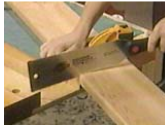
Cut off any bad ends and then cut the boards to length
